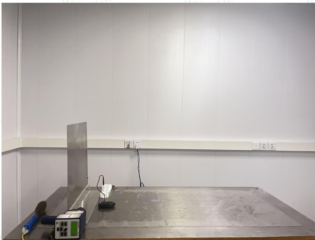
Test Setup Photo of Electrostatic Discharge Test
