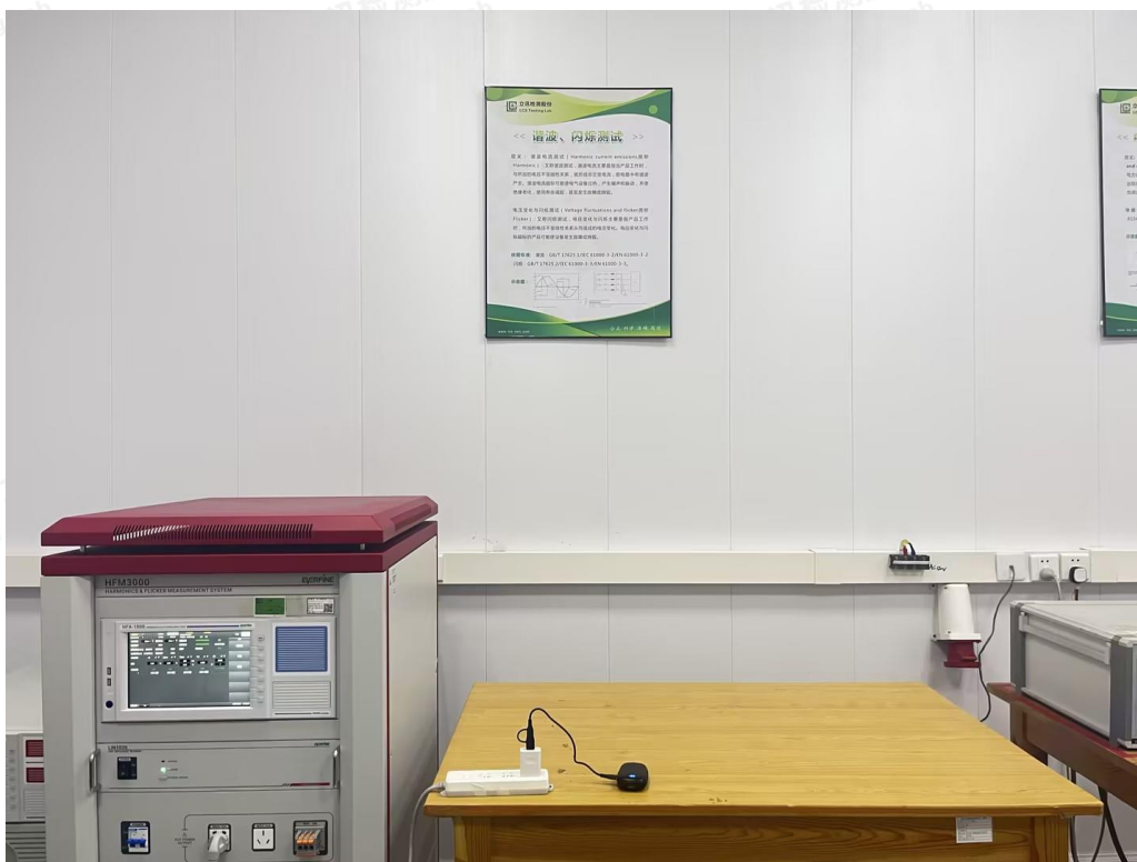
Test Setup Photo of Harmonic &amp; Flicker Measurement
