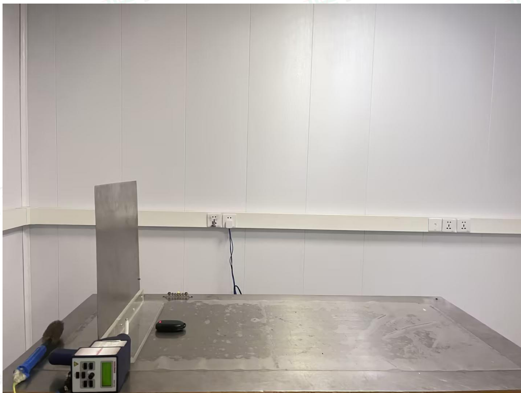
Test Setup Photo of Electrostatic Discharge Test
